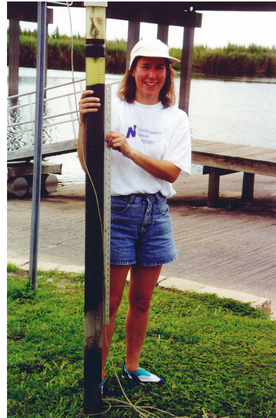
Figure 1. This sediment core from Lake Jesup, Seminole Co., Florida, represents more than 100 years of depositional history. A coring device of this size permits all analyses to be performed on material from a single core.
